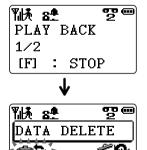
3 Press FISELECT to delete, or turn the Easy Shuttle to select "NOT DELETE" and press FISELECT to leave.
